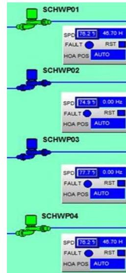
Figure 5. Post RCx SCHW Pumps only 2 running
